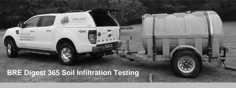
Soakage tests are required in order to determine the infiltration rate and drainage capacity of the soils. This will aid the design or indeed rule out the suitability of soakaways.
