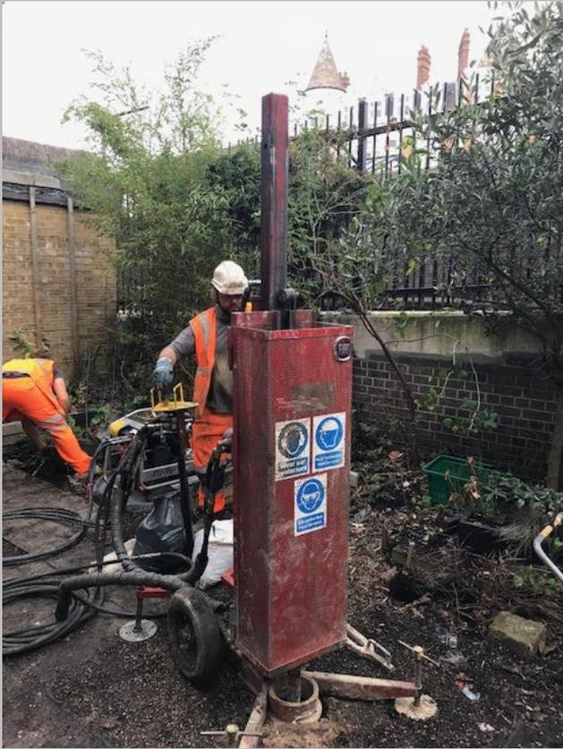
Our modular windowless sampling equipment is ideally suited to sites where only narrow access is available; the wheel mounted mast with drop hammer unit can be wheeled through small openings. With hydraulic quick connectors and extension hoses, the drill unit can be used remotely up to 30m from the base unit. The system is equipped with a PTO to connect other hydraulic tools including concrete corers, small breakers, etc.
