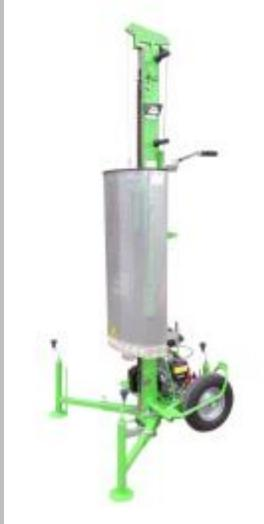
The Geotool dynamic probing rig is a versatile, lightweight option for working in more restricted sites. It is driven by a Honda GX100 petrol engine with three legs for stability. Both dynamic probing and driving window sample tubes can be achieved with adaption for different drop weight masses (10, 30, 50, 63.5kg) by removal or addition of weights meaning that DPL, DPM, DPH and DPSH as well as SPT can be carried out. The drop weight carriage is lifted and lowered on the mast with an
