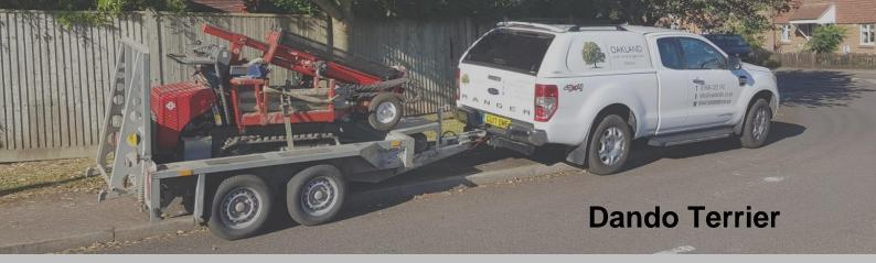
The ultra-small, compact Dando Terrier rig has been designed specifically for sampling and testing for geotechnical and environmental analysis and is crawler mounted for easy site access in difficult conditions.
