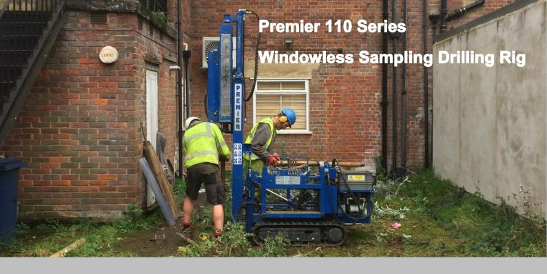
Engine - Honda 13hp GX390 petrol engine with electric start
